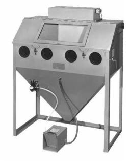
NEVER USE SILICA-BASED PRODUCTS IN TRINCO™BLAST SYSTEMS Ref. NIOSH Alert # 92-102
